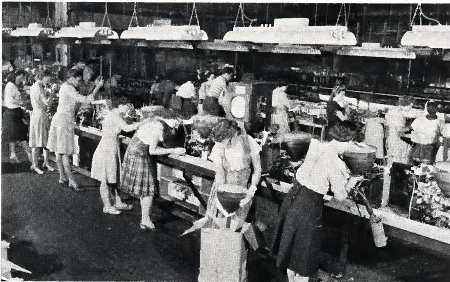
The Camden assembly line checking 10-inch direct viewing tubes for RCA's television table model receivers now in production. Set has 13-channel tuning, television only.
